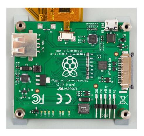
Using the white ribbon cable supplied, connect one end to the controller board, **making sure that this end has the blue tab facing down**, towards the board (the opposite end, the end not being attached to the controller board, should have the blue tab facing up, so you can see it):
