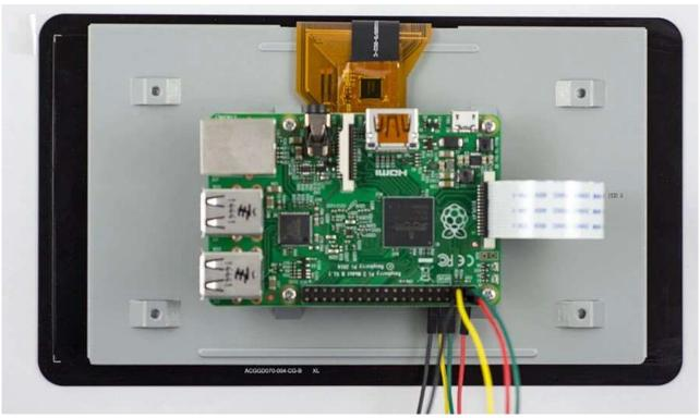
Now it's time to power it all. Plug an official Raspberry Pi power supply into the controller board (the controller board will power your Pi via the jumper wires) and away you go!).
