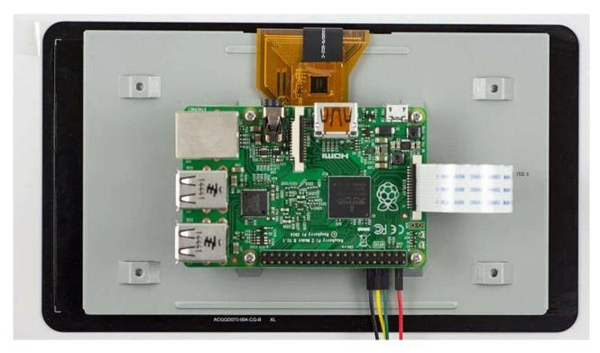
Now connect the jumper wires to the Pi. Again, only the black and red wires are required.
