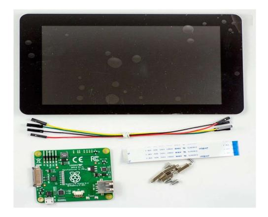
Start by connecting the large ribbon cable from the screen to the connector on the underside of the controller board. You will need to carefully undo the clamp before inserting the cable. Make sure to press the clamp in to secure the ribbon in place.
