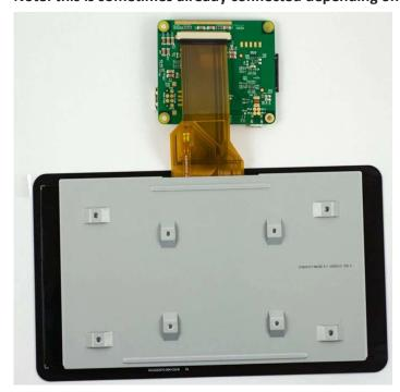
Now turn the controller board over, and connect the small ribbon cable from the screen to the board. Same principle as above, undo the clamp, insert cable, press clamp closed to secure ribbon in place.
